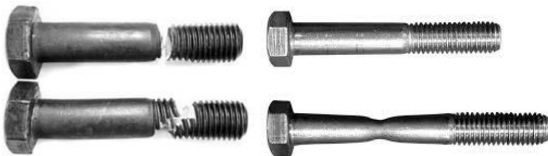
Figure 5: Bolt Fracture [8] (left), Plastic Deformation [9] (right)
