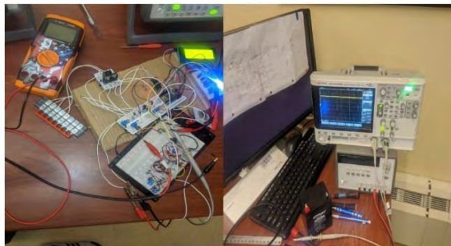
Figure 15: Testing the Charge Controller Circuit
