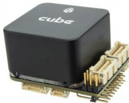
Figure 1: Pixhawk Cube on Mini Carrier Board.
