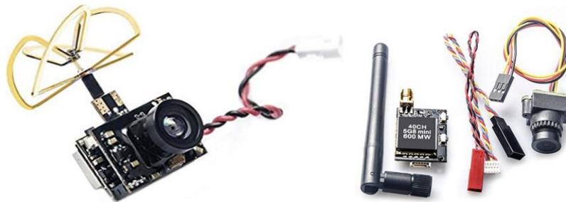
Figure 6: Camera with FPV Transmitter
