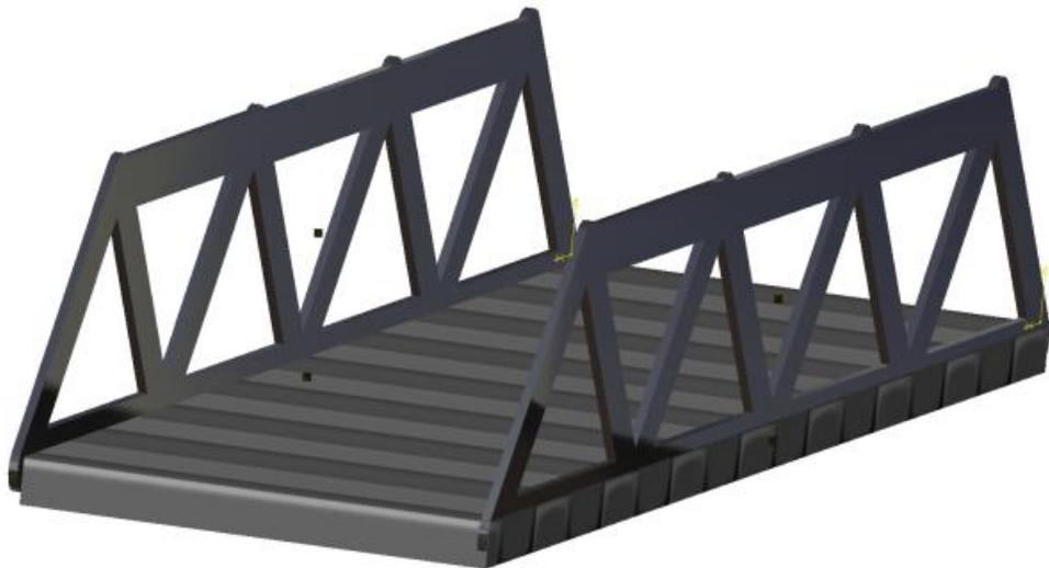
**Figure 1: CATIA design of a Warren truss bridge**
