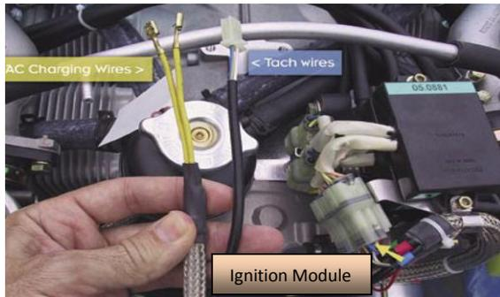
Figure 3. External Electrical Modules Lockwood, 2004)
