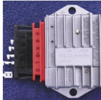
Figure 4. Rectified-Regulator-Filter Module (Lockwood, 2004)
