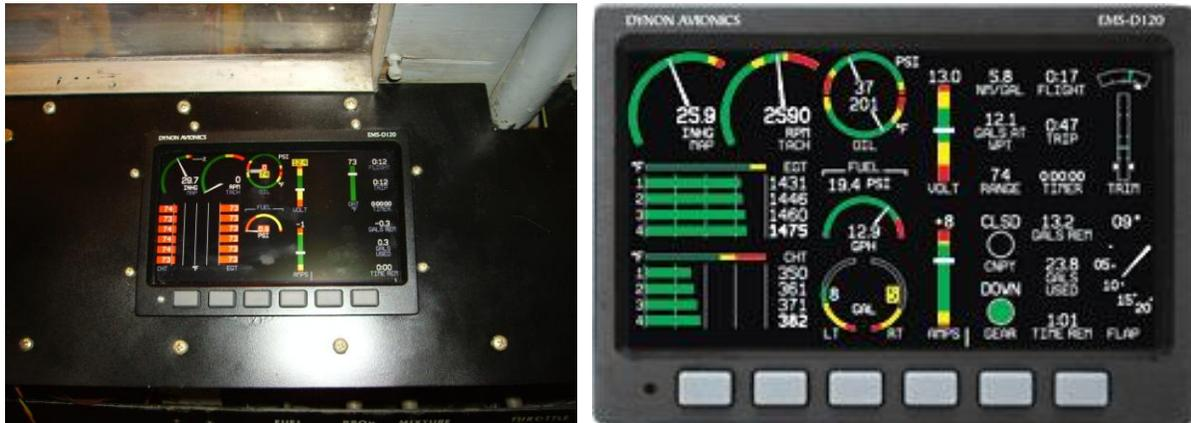
Figures 6 and 7. Depiction of Dynon EMS-D120 display with engine off and engine running (Hannon and Harrison, 2009)
